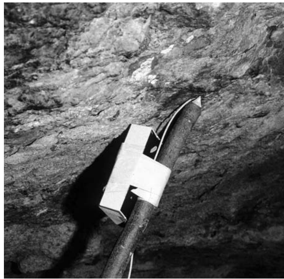
Figure 1a (top). Thermocouple located with chisel pointed branch. Figure 1b (above). Thermocouple and co-located relative humidity sensor.
